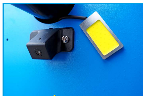
LASER INDICATOR AND WHEEL INTERIOR LIGHTING
